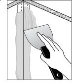
knife press the tape into the corner. Use enough pressure to squeeze some compound from the edge of the tape, but leave enough compound to form a good bond. Feather the compound 2" (51 mm) from the edge of the tape. Let dry 24 hours, finishing only one side at a time. Let dry, finish other side of corner. Let dry, then sand corner. Be careful not to let the compound build up in the very corner of the tape. Excess compound in the corner could cause hairline cracks.
